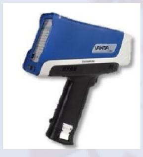
The Vanta analyzer is our most advanced handheld X-ray fluorescence (XRF) device and provides rapid, accurate element analysis and alloy identification to customers who demand laboratory-quality results in the field.
